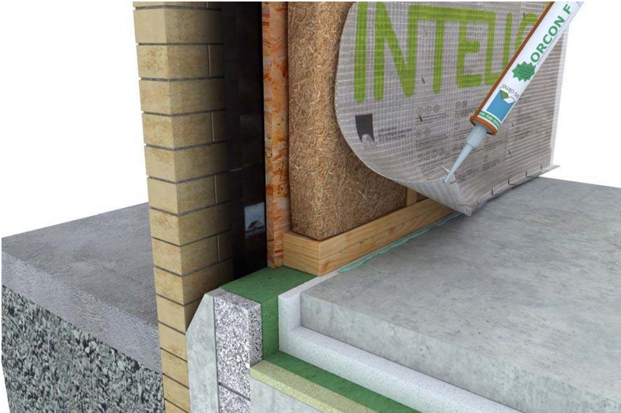
Figure 1: Bonding of Intello Plus to Concrete Slab using ORCON F
