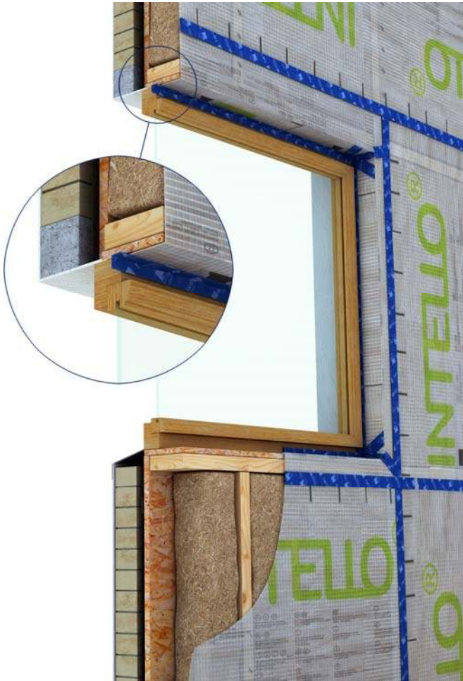
Figure 2: Window Detail sealed with TESCON PROFIL
