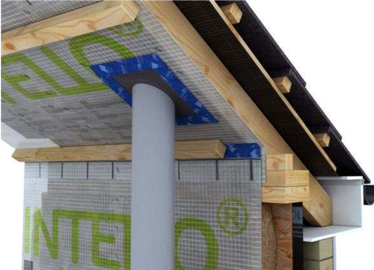
Figure 4: Roof Detail with Pipe Grummet
