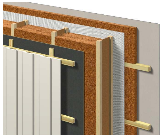
Fig. 1 Illustration of principle of Hunton wall
